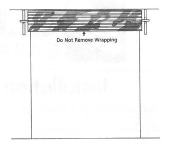
Tension should now be applied to the spring by rotating the door about 1½ times in a forward direction, as shown. The amount of tension required to give the best operation may vary with individual doors. Final adjustment should be made on completion of the job.
